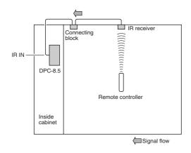
Connect the IR receiver to the DPC-8.5 as shown below.
